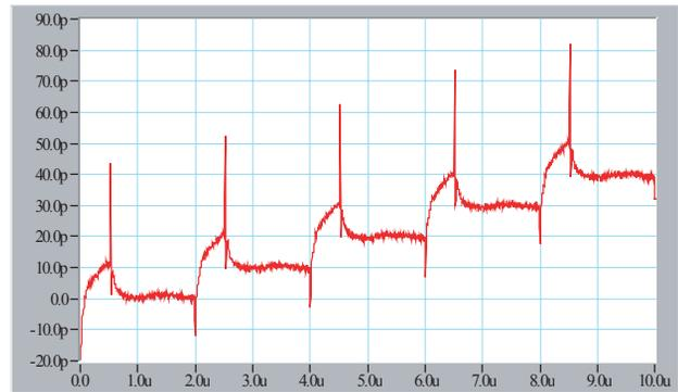
Figure 4: ~9.8pC steps for 2us spacing.
