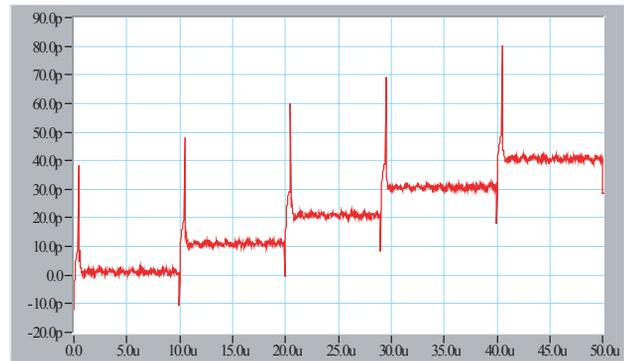
Figure 3: 10pC steps for 10us spacing.
