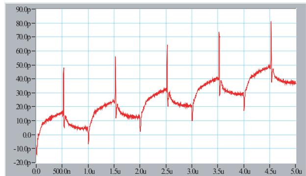
Figure 5: ~8pC steps for 1us spacing.
