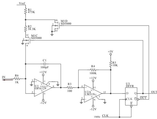
Figure 2: Simplified Recycling-Integrator Schematic.
