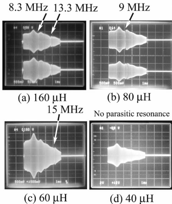
Figure 4: Dependence of the parasitic resonances on the anode inductance, (a) 160  $\mu$ H, (b) 80  $\mu$ H, (c) 60  $\mu$ H and (d) 40  $\mu$ H. Envelopes of two gap voltages are shown separately in (a) and (b), but their difference is given in (c) and (d). The horizontal axis is 1 ms/div.
