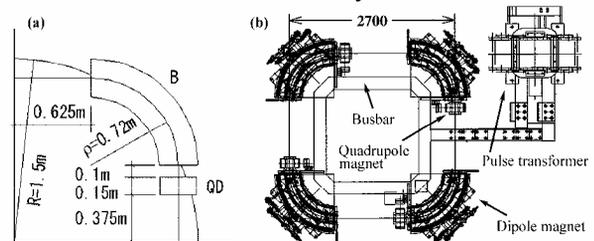
Figure 1: (a) DOB lattice and (b) the assembled image of the ring.
