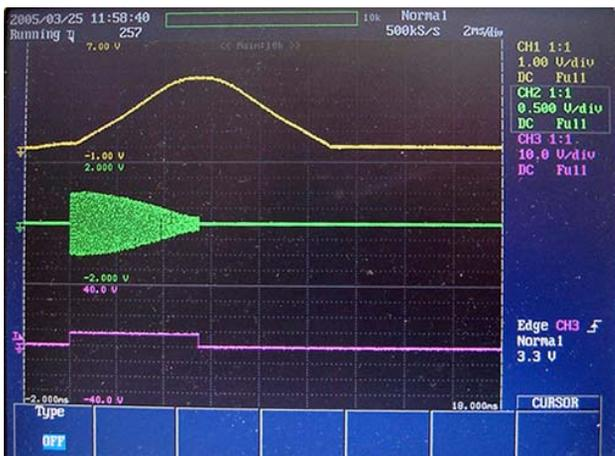
Figure 5: Performance of the real-time acceleration voltage feedback. Top: Dipole current waveform, Middle: Envelope of the programmed gap voltage, and Bottom: Gate signal to the RF amplifier.
