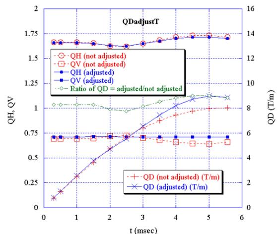
Figure 2: Example of the fine tuning for DOB lattice. In this case the current pattern of QD is controlled so that the vertical tune QV is constant during acceleration. The filled squares and circles are after the fine tuning and the corresponding QD excitation is marked with the symbol "x".
