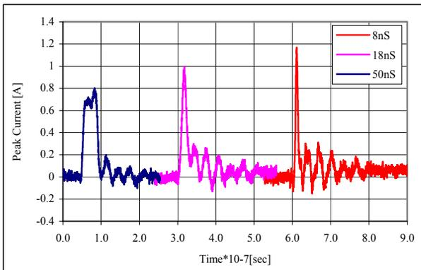
Figure 4: Toroid output for the 40nS, 18nS, and 8nS FWHM electron beam pulses.
