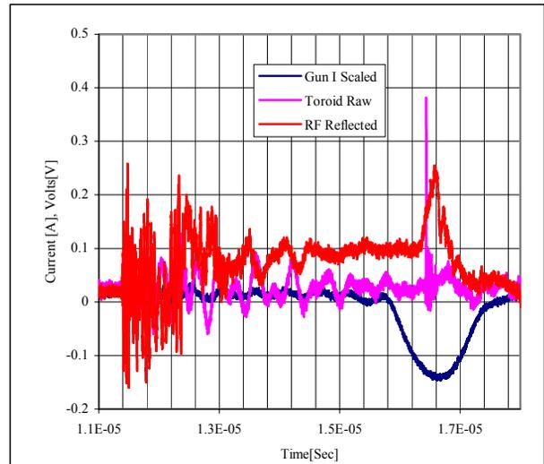
Figure 2: Scaled gun current pulse, reflected RF signal and raw toroid for 8nS FWHM electron pulse.
