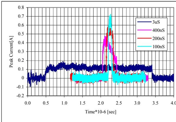
Figure 3: Toroid output for the 3uS, 400nS, 200nS and 100nS FWHM electron beam pulses.
