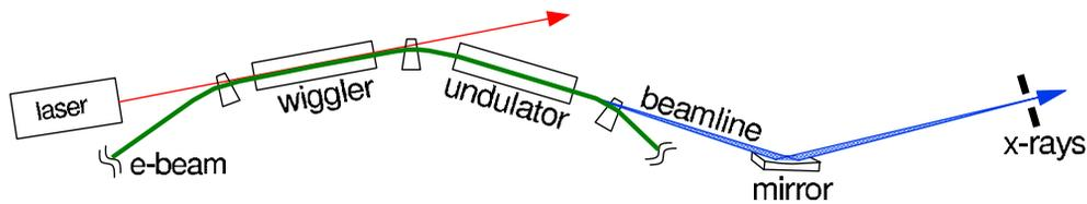
Figure 1: Sketch of slicing arrangement at ALS.
