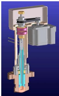
Figure 3: Beam aperture defining collimator used to locate beam losses away from the in-vacuum undulator.
