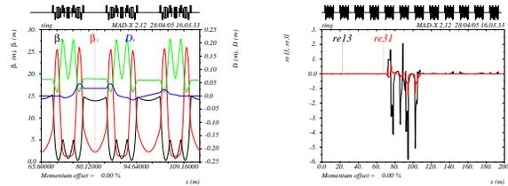
Figure 4: Lattice functions and coupling angles for the new dispersion bump using 12 instead of 4 skew quadrupoles. Global coupling as well as local coupling in the in-vacuum undulator straight are very small.
