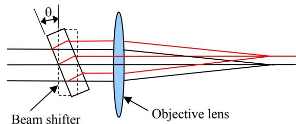
Figure 6: Function of beam shifter for the calibration of beam position by sifting the input optical axis.
