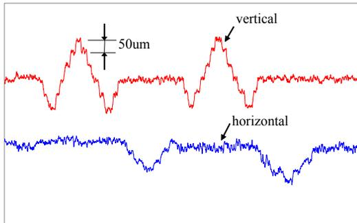
Figure 7: Result of calibration for beam positions. One step of the calibration corresponds to 50 $\mu$ m.
