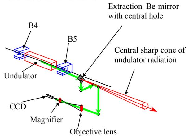
Figure 1: Layout of optics system of the monitor.
