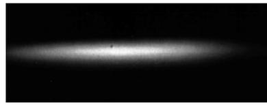
Figure 4: Separated beam image in the BL-5 undulator. The gap of undulator is 140mm.
