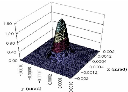
Figure 2: Power distribution of radiation from BL-5 undulator. The gap of undulator is 70mm.
