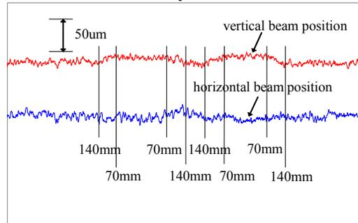
Figure 8: A result of measurements beam positions during moving the gap from 140mm to 70mm.
