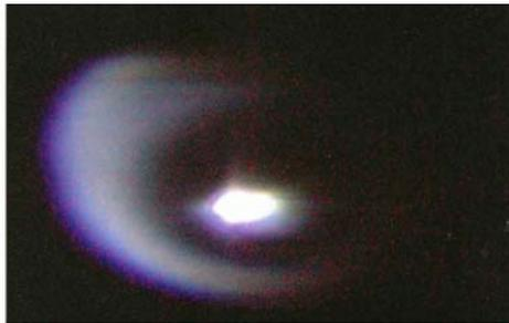
Figure 3: image of undulator light (central bright spot ) with defocused bending light from the downstream bending magnet.
