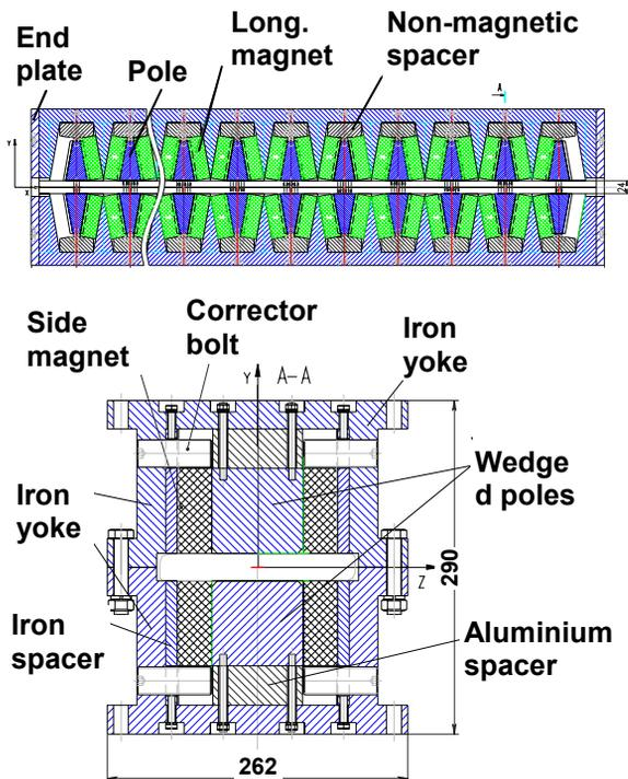
Figure 3: Longitudinal and transverse wiggler cross sections.
