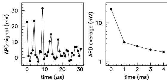
Figure 6: Time-resolved APD signal from successive turns (left) and on the millisecond time scale (right). After 1 ms, the betatron motion is no longer visible and the signal was averaged over several turns.
