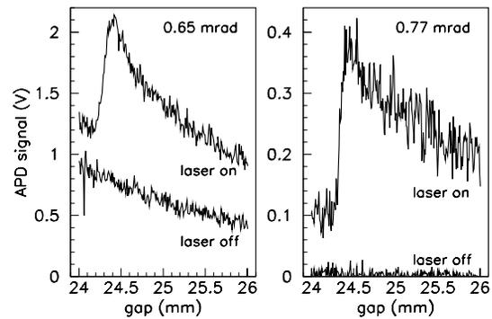
Figure 5: Femtosecond x-ray signal and background (laser off) at 708 eV as function of the UE56 magnetic gap for two observation angles, scanning the 3rd undulator harmonic.
