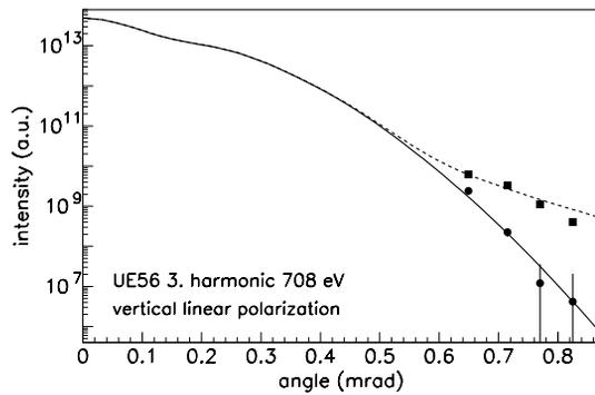
Figure 4: Calculated (lines) and measured (dots) angular distribution of synchrotron radiation at 708 eV with vertical linear polarization with and without energy modulation.
