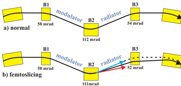
Figure 3: Sketch of the electron orbit for (a) normal operation and for (b) femtoslicing, where low-energy electrons (blue arrow) are aligned with the radiator axis and radiation from the bend magnets B2 and B3 misses the beamline.
