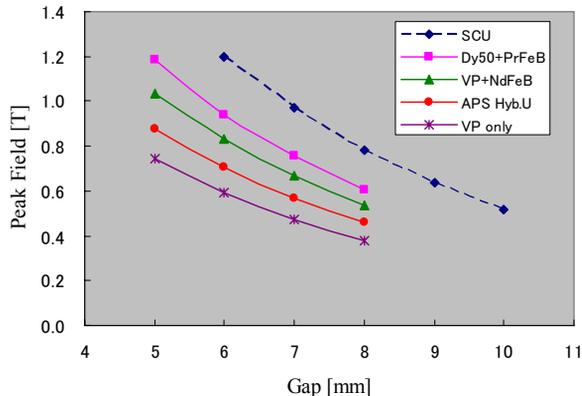
Figure 7: Peak field as a function of gap for various devices.
