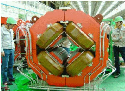
Figure 5: A large-bore quadrupole magnet for the 3-GeV RCS.
