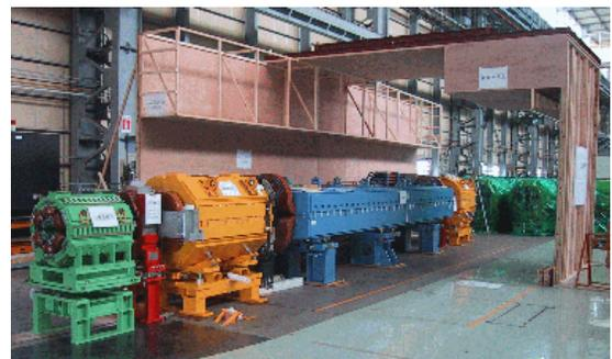
Figure 8: Mock up of the MR tunnel. Bending, Quadrupole and Sextupole magnets are in blue, orange and green, respectively.
