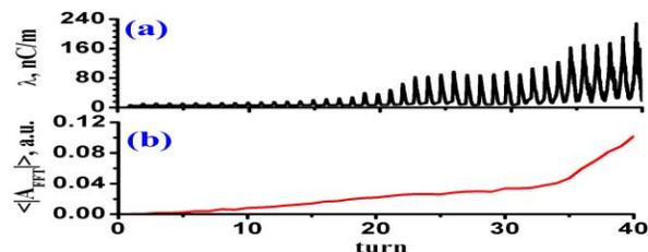
Figure 1: Instability development for variant 1 in Table 1. (a) – linear electron cloud density; (b) – average amplitude of the vertical beam oscillations.
