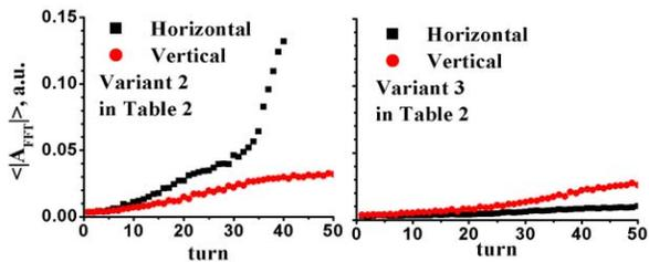
Figure 4: Effect on instabilities in both planes when the ECNs inserted into dipole magnets.
