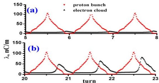
Figure 3: The electron cloud and proton bunch linear densities as functions of time (turn number). (a) - turns 5-8. (b) – turns 20-23.
