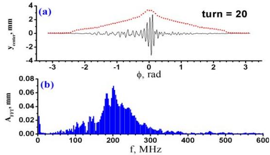
Figure 2: The proton bunch at turn 20. (a) – vertical oscillations as function of longitudinal phase with longitudinal profile. (b) – a frequency spectra.
