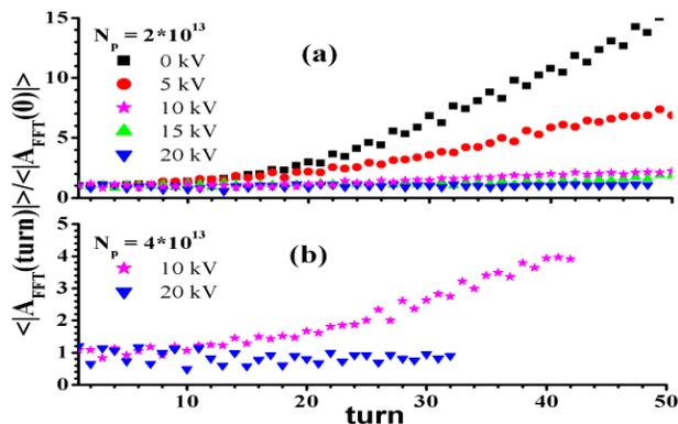
Figure 5: The time evolution of average amplitudes of the vertical proton beam oscillations. (a) – 3.2  $\mu\text{C}$  and (b) - 6.4  $\mu\text{C}$  cases.
