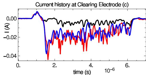
Figure 3: Current history at clearing electrodes (a), (b) and (c): red - recorded on HCX experiment, black - WARP simulation with secondary electrons OFF, blue - WARP simulation with secondary electrons ON.
