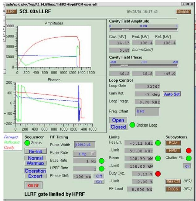
Figure 1: Low Level RF traces of forward (blue), reflected (green) and transmitted (red) amplitude (above) and phase (below) for a SNS superconducting cavity.
