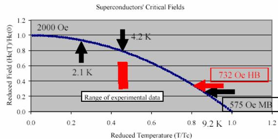
Figure 3: Theoretical magnetic field limits for a superconductor as a function of temperature. The operating values for SNS are well below the theoretical limits (blue curve).
