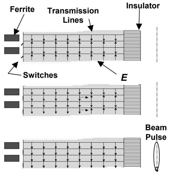
Figure 1. Symmetric Blumlein operation. Top: charging cycle. Middle: switches close to generate reverse polarity wave. Lower: beam injected and accelerated until transmission line is discharged. Ferrite isolates the leakage current resulting from the unswitched line.
