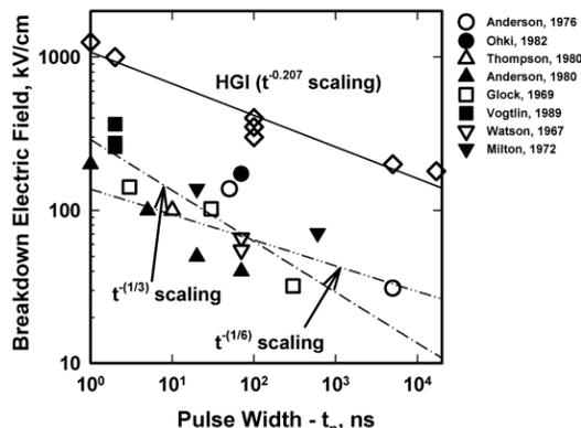
Figure 3. Comparison of multilayer HGI structures with conventional 0° insulators.
