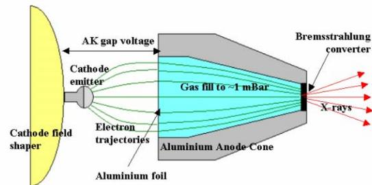
Figure 5: Paraxial Diode.
