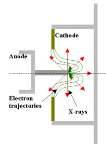
Figure 4: Rod Pinch (Positive Polarity).
