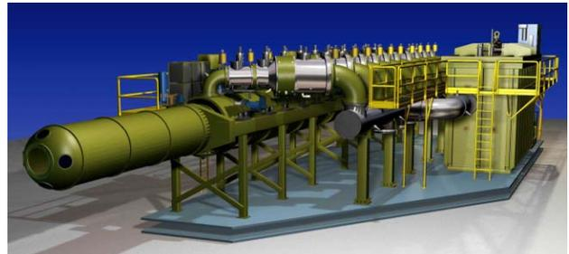
Figure 9: The 10 stage IVA for new AWE radiographic facilities.
