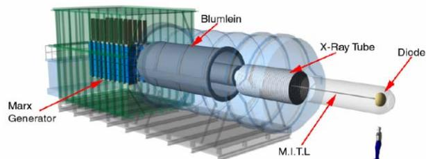
Figure 2: The Single (Blumlein) Pulse Forming Line Pulsed Power Machine.
