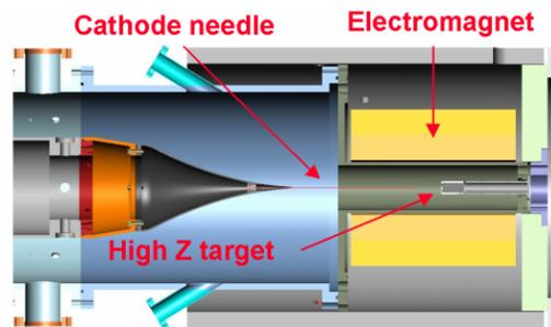
Figure 6: Immersed B Field Diode
