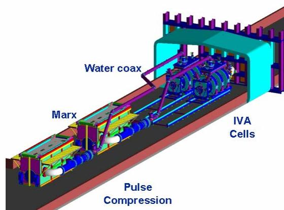
Figure 8: The two CYGNUS IVAs as configured at the NTS.
