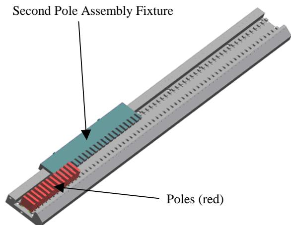
Figure 5: Long magnetic structure with second pole assembly fixture.
