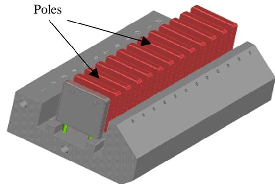
Figure 2: Current LCLS magnetic structure design (poles and base only).
