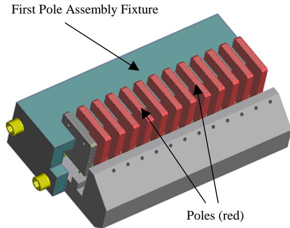
Figure 3: Magnetic structure with the first pole assembly fixture.
