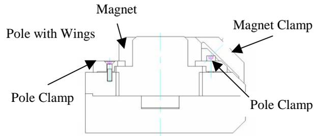
Figure 1: Initial LCLS magnetic structure design.
