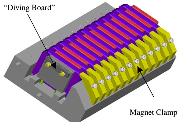
Figure 4: Fully assembled short magnet structure.
