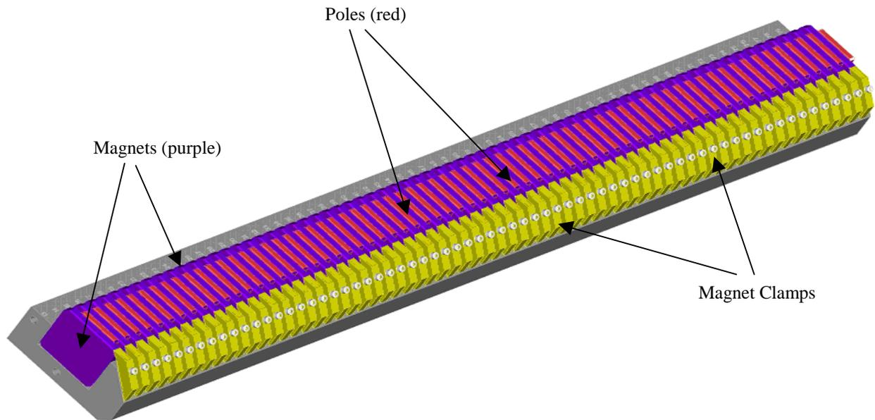
Figure 6: Fully assembled long magnet structure.
