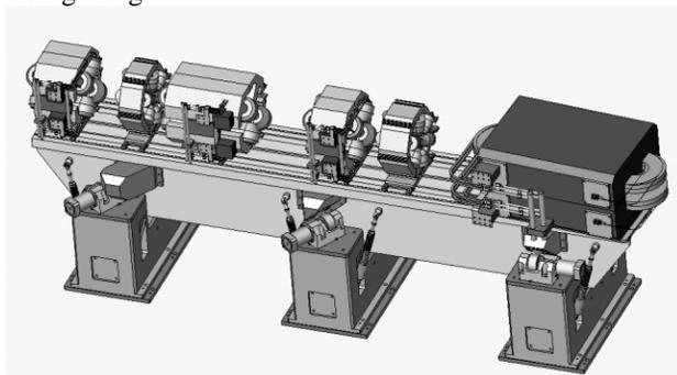
Figure 1: Schematic diagram of the magnets installed in the storage ring.
