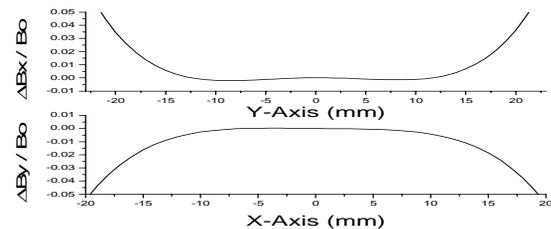
Figure 7: The calculated field distribution of the horizontal and vertical steering coils in the sextupole magnet.
