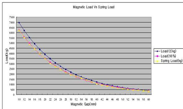
Figure 5: Magnetic load and spring load Vs magnetic gap-dependent
