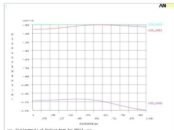
Figure 3: ANSYS results for the backing beam in the vertical (y) direction along Z-direction (beam pass) of backing beam at no load, maximum magnetic load and maximum magnetic load with reaction force.
