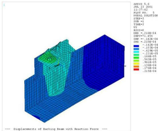
Figure 4: ANSYS result for the backing beam in the vertical (y) direction. The maximum deformation is about 21.60  $\mu\text{m}$  if 14 metric tons of magnetic load and reaction force with magnetic load compensation spring system are applied.
