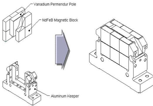
Figure 1: Geometry configuration of half period
