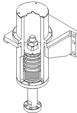
Figure 6: Design of magnetic load compensation spring system
