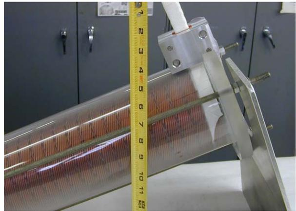
Figure 2: Pulsed solenoid ready for first potting
