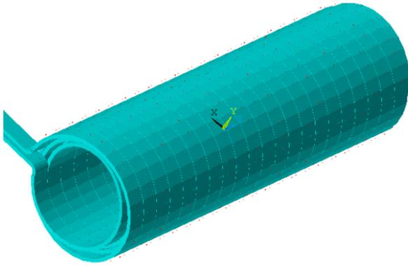
Figure 1: Pulsed Solenoid Finite Element Model
