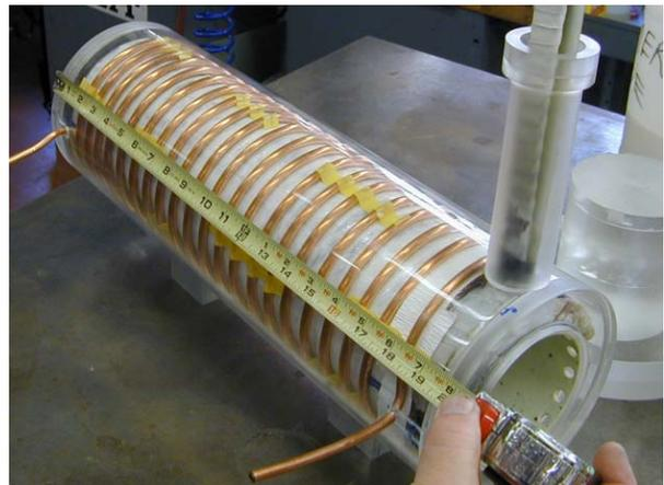
Figure 3: Pulsed solenoid ready for final potting
