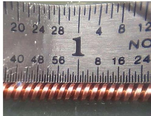
Figure 4: Windings enlarged. Scale in minimal division is 1/64 of an inch.
