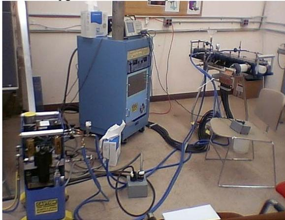
Figure 5: Testing setup. Visible are undulators at the right, pulser at center and cooling system at the left.
