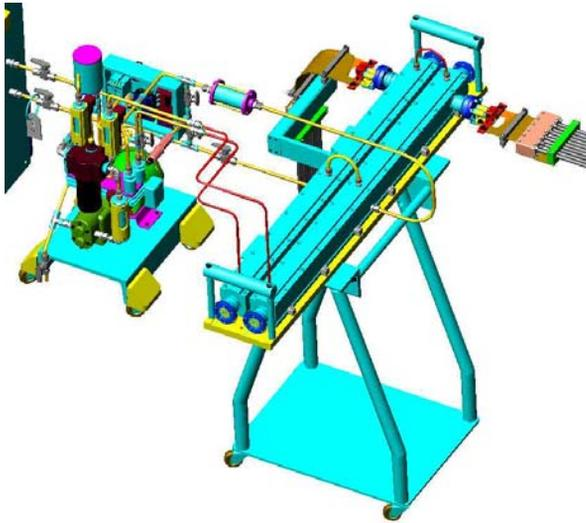
Figure 3: Set of two undulators installed on platform shown with cooling system, left. The last one shown with cover removed for better visibility.
