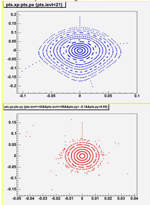
Figure 5: x vs.  $P_x$  and y vs.  $P_y$  phase space plots illustrating how the dynamic aperture is calculated. The spacing between initial muon trajectories is 1 cm.
