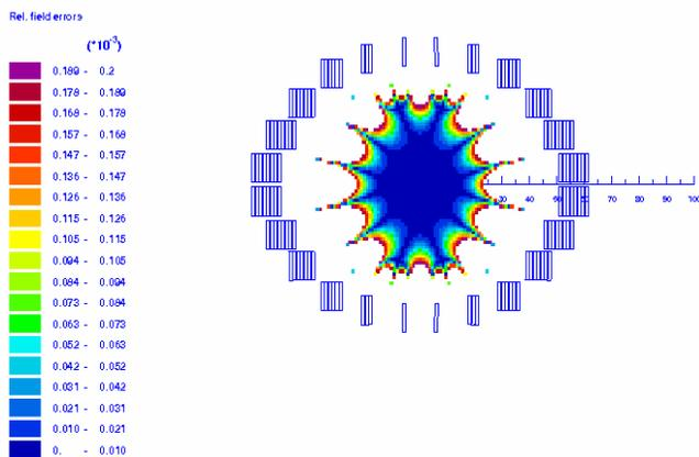
Figure 4: 2-D field quality computation of an alternative coil arrangement, investigated to design a curved dipole magnet
