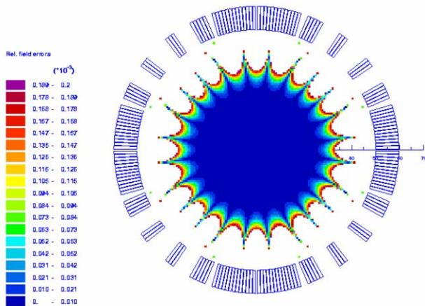
Figure 2: 2-D field quality computation of the HESR quadrupole.
