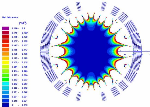
Figure 1: 2-D field quality computation of the HESR Dipole done with ROXIE[4]
