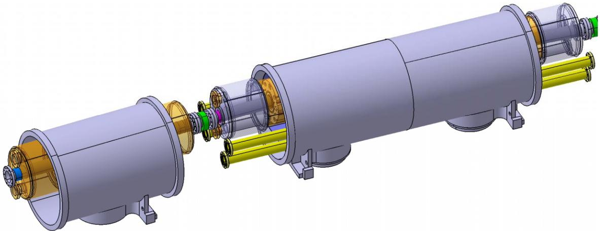
Figure 3: Three-dimensional view of a dipole and the adjacent quadrupole magnet of the HESR ring.
