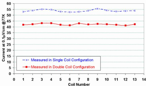
Figure 3: The current at an average voltage gradient of  $0.1 \mu\text{V}/\text{cm}$  ( $10 \mu\text{V}/\text{meter}$ ) over the total length of the coils measured at  $77 \text{ K}$  for the first thirteen pancake coils powered individually and in pairs.
