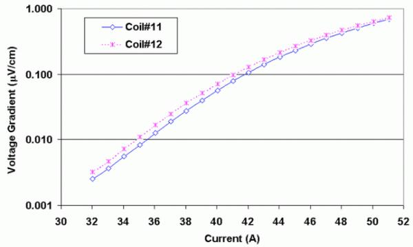
Figure 4: Typical voltage gradient vs. current curves for a pair of coils operated in series in liquid nitrogen bath.
