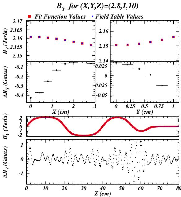
Figure 4: Residuals of the analytic description of the vertical component of the wiggler field.
