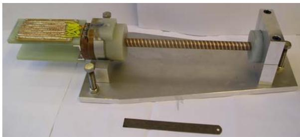
Figure 5: Undulator prototype completed.
