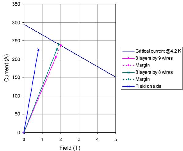
Figure 3: Undulator conductor load lines.
