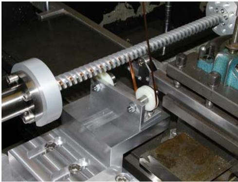
Figure 4: Undulator winding on a lathe.
