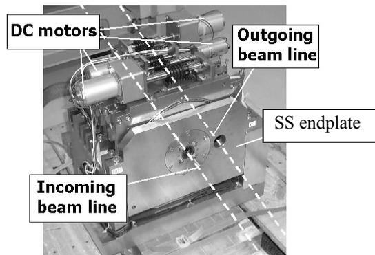
Figure 2: Fabricated adjustable PMQ.
