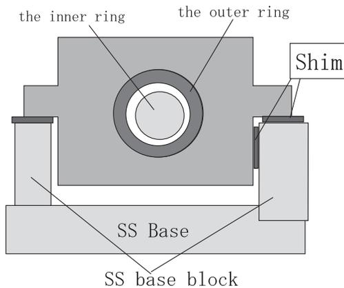
Figure 7: Sketch of PMQ showing shim placement.
