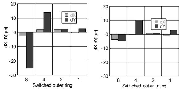
Figure 8: Center Movement affected by shimming. Left: Before shimming. Right: 8cm ring lifted up by 76μm. "8" means 8cm long outer ring.
