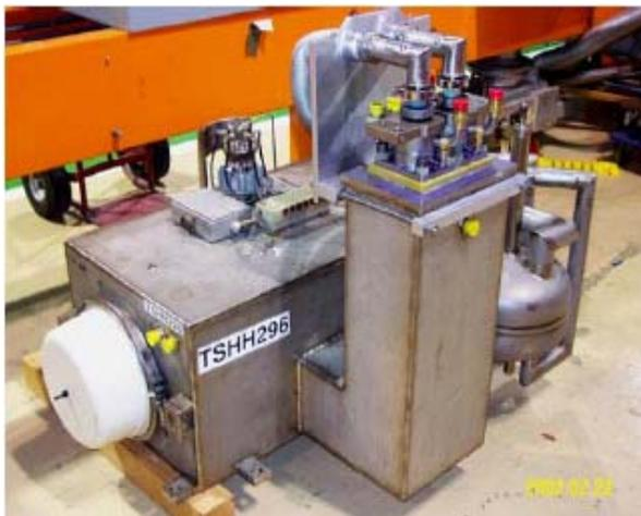
Figure 1: Standard Tevatron spool with HTS leads.
