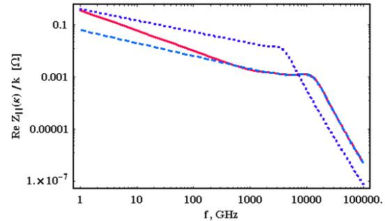
Figure 3: Distribution of the real part of transverse dipole mode (solid). Also shown: copper (dashed) and stainless-steel (dotted) tubes truncated impedances.
