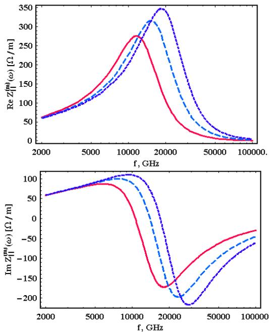
Figure 2: Distributions of real (top) and imaginary (bottom) parts of the longitudinal modes for  $m=1$  (solid), 2 (dashed) and 3 (dotted) for SS-copper tube.
