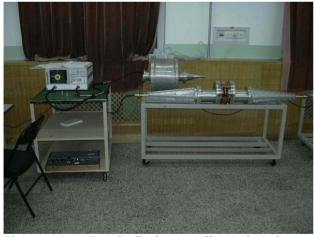
Figure 1: Longitudinal coupling impedance measurement platform for BEPCII.
