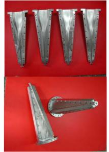
Figure 2: Gradual change impedance matching sections. Upper for inside face and lower for assembled parts.
