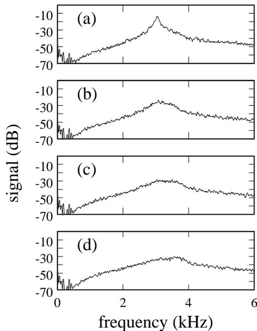
**Figure 4.** Experimental phase noise at a ring current of 150 mA, when an Agilent E4400B signal generator is used as the master oscillator. (a) Robinson dipole feedback off. (b) Robinson dipole feedback gain 12 dB below maximum. (c) Robinson dipole feedback gain 6 dB below maximum. (d) Maximum Robinson dipole feedback.
