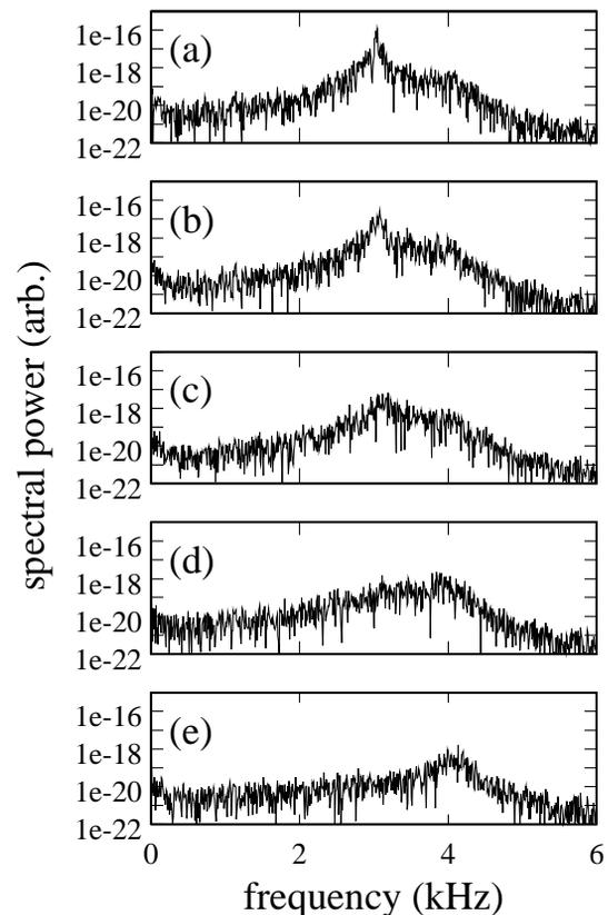
**Figure 3.** Spectral power in simulations of Robinson dipole feedback for a current of 150 mA. (a)  $\tau_{\text{feedback}} = 10$  ms. (b)  $\tau_{\text{feedback}} = 3$  ms. (c)  $\tau_{\text{feedback}} = 1$  ms. (d)  $\tau_{\text{feedback}} = 0.3$  ms. (e)  $\tau_{\text{feedback}} = 0.1$  ms.
