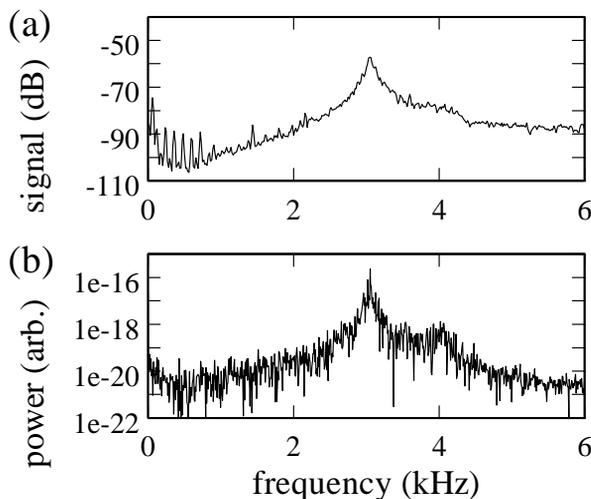
**Figure 2.** (a) Experimental spectrum of phase noise for standard double-hump bunches with a current of 144 mA, when an Agilent E4400B signal generator is used as the master oscillator. (b) Spectral power density of the average bunch centroid position in a 500,000-turn simulation.
