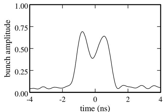
**Figure 1.** Data from the Q-electrode show the double-hump bunch shape during standard operation of the LF15 low-emittance lattice. Effects of the Q-electrode capacitance and cable dispersion have been corrected by software.
