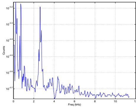
Figure 3: A steady-state closed-loop LER beam spectrum measured at 2050 mA via the LFB system
