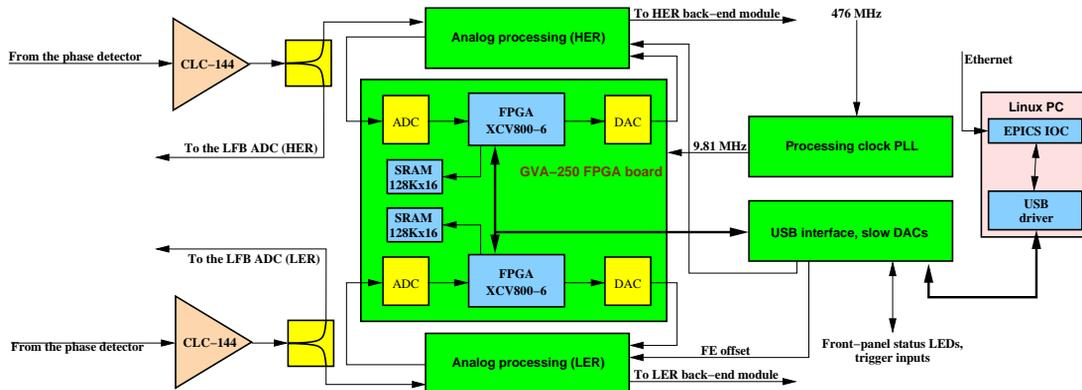
Figure 1: A block diagram of the low group-delay woofer
