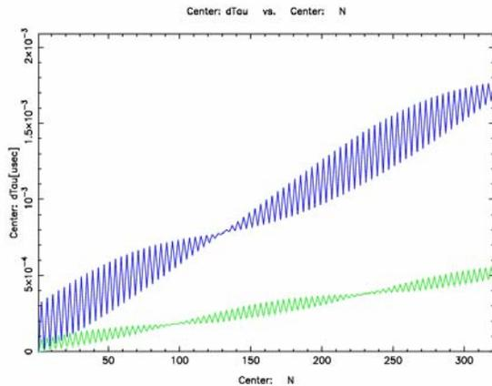
Figure 5: As function of the number of turns  $N$ ,  $\delta\tau$  [ $\mu\text{sec}$ ] is plotted, the deviation of the ToF of the two ions that are closest to the optical axis in Figure 4 relative to that of a reference ion.
