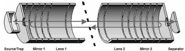
Figure 1: Sketch of the multi-pass time-of-flight mass separator that consisting of coaxially arranged electrostatic mirrors and lenses built as ring electrodes. Further downstream a fast ion separator selects ions of a certain mass.
