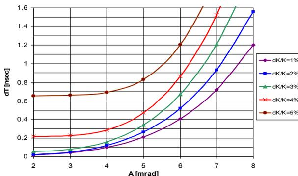
Figure 6: The MTOF time spread per turn versus beam r.m.s. angle  $\pm A$  for different r.m.s. energy spreads  $\delta=\pm dK/K$  and r.m.s.  $X=\pm 1.5\text{mm}$ . (Beam energy  $K=1.5\text{kV}$ , mass  $A=100\text{ a.m.u.}$ , period  $T_0=51.8\mu\text{s}$ .)
