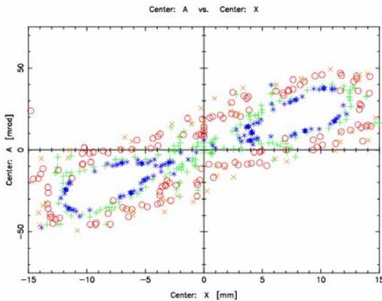
Figure 3: Motion of ions in the phase plane a[mrad]-x[mm] at  $Q$  close to 0.5. All shown ions are unstable and lost after less than 100 turns.
