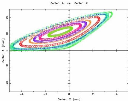
Figure 2: Stable motion of ions in the phase plane a[mrad]-x[mm] around the 1<sup>st</sup> order fixed point. The tune  $Q$  is close to 1.0, number of turns  $N=320$ .
