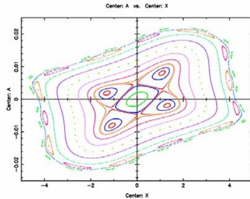
Figure 4: Motion of ions in the phase plane a[rad]-x[mm] for tune  $Q=0.73$ . Number of turns  $N=2000$ . The shown stable area is around  $80\pi$  mm\*mrad.
