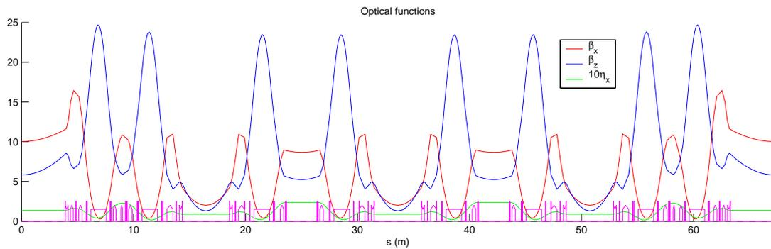
Figure 1: Optical functions for a quarter of the machine. All the units are in meters.
