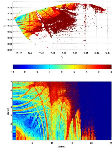
Figure 5: Frequency map for a sample machine, including closed orbit errors and correction.
