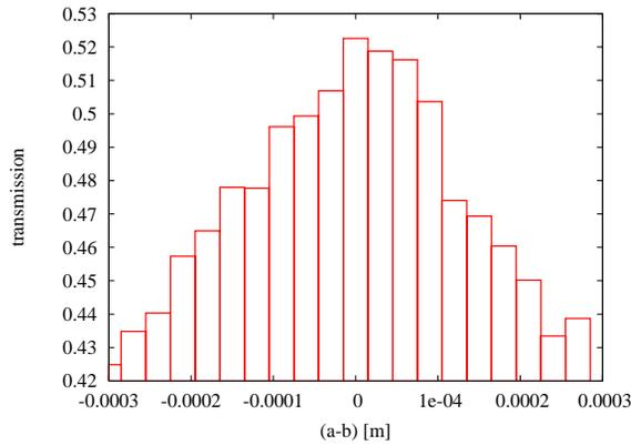
Figure 2: Simulated result of alignment scan. The maximum of the curve corresponds to the maximum achievable collinearity between beam and jaw.
