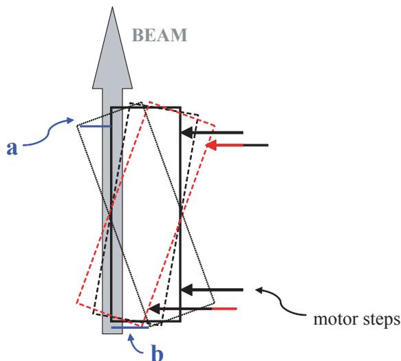
Figure 1: An illustration of the alignment scan. Both jaw ends are moved by the same amount of steps in opposite directions.
