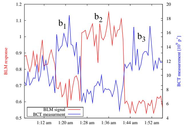
Figure 5: BLM and BCT signals during scraping with the collimator.
