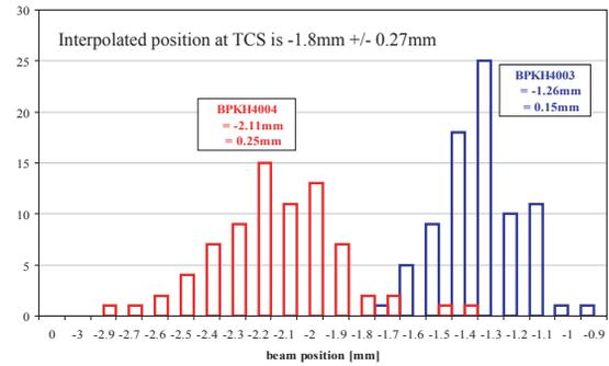
Figure 3: The results of the BPM measurements to define the beam position at the collimator.
