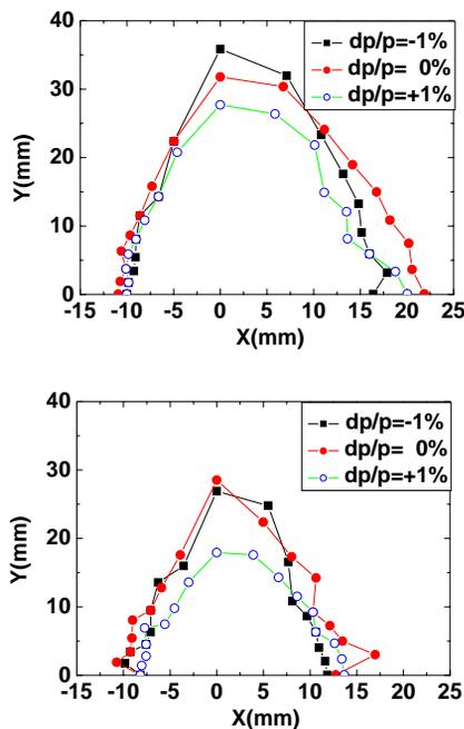
Figure 5: Dynamic apertures in the lattice with the emittance of 10.3 nm. (Top) Without machine errors, (bottom) with machine errors.
