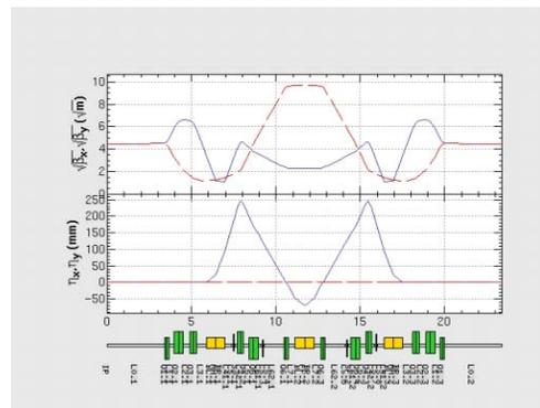
Figure 6: A designed lattice for the quasi-isochronous mode in 2.5 GeV ring. Momentum compaction factor is  $6.8 \times 10^{-6}$ .
