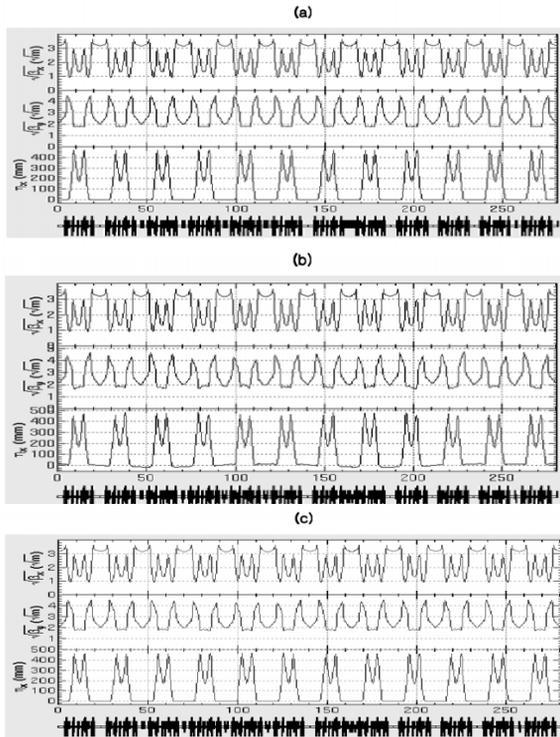
Figure 2: Optics at the 2.5 GeV ring: without the insertion devices, (b) with the six insertion devices, and (c) with the six insertion devices and optics compensation.
