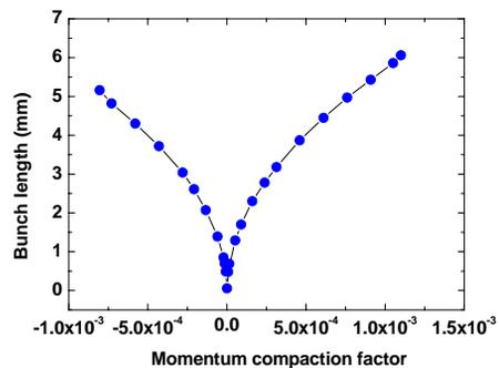
Figure 7: Rms bunch length as a function of the momentum compaction factor in the 2.5 GeV ring.
