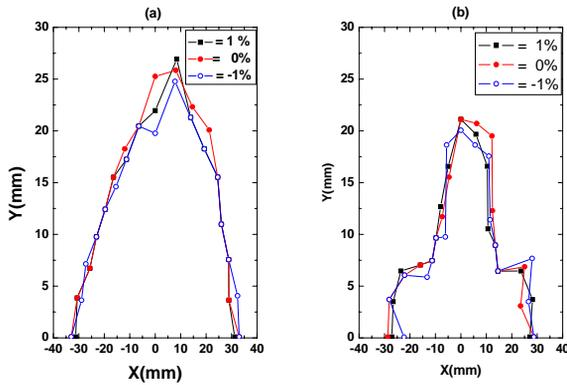
Figure 1: Dynamic apertures at the center of the straight section: (a) without the insertion devices ( $\nu_x = 14.28$  and  $\nu_y = 8.18$ ) and (b) with the six insertion devices ( $\nu_x = 14.28$  and  $\nu_y = 8.237$ ).
