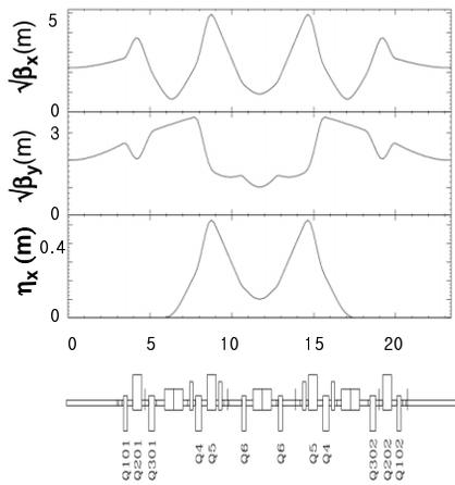
Figure 4: A lattice with emittance of 10.3 nm at 2.5 GeV.
