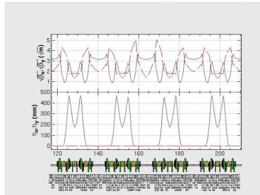
Figure 3: A designed lattice for low-beta in the In-vacuum undulator at 10th cell in the ring. Vertical beta-functions (red one) with a low-beta and with normal-beta in the straight sections are 2 m and 4 m, respectively.
