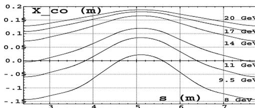
Figure 3: Closed orbits at various energies.
