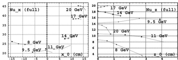
Figure 7: Amplitude detuning and its energy dependence.
