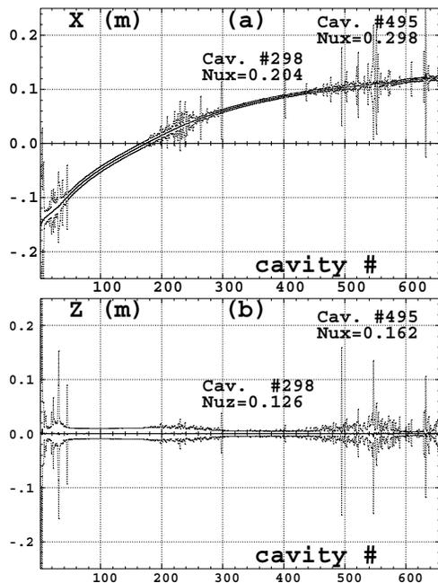
Figure 9: Beam centroid position and envelopes.
