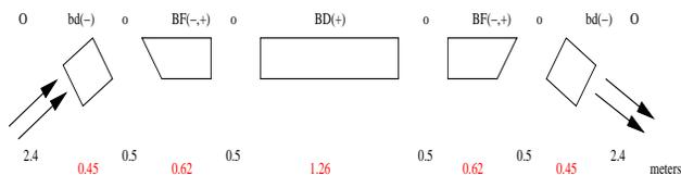
Figure 1: Isochronous cell.
