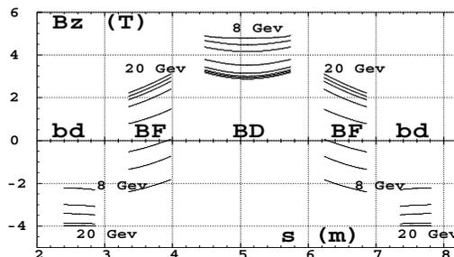
Figure 2: Magnetic field on closed orbits at various energies.
