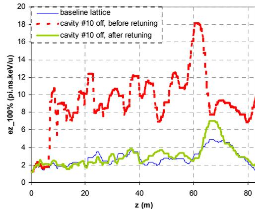
Figure 4: Longitudinal emittance along the first linac segment for  $U^{28,29+}$  beam. The loss of a single cavity in the early part of the segment can lead to severe mismatch and phase space distortion if no cavity retuning is applied. After retuning, the performance of the segment is usually recovered.
