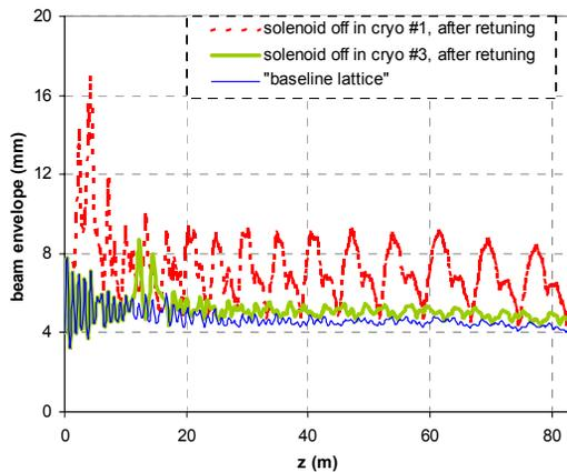
Figure 3: Beam envelopes of  $U^{28,29+}$  beam for unperturbed lattice (blue) of Segment I, and for lattices with a single solenoid failure in Cryomodules No. 1 (red) and No. 3 (green).
