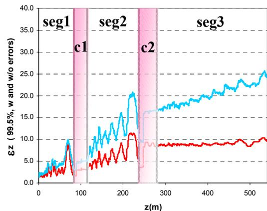
Figure 2: Longitudinal emittances of multi-charge state uranium beam w/o errors (red/dark) and with errors (blue/light) along the RIA driver linac.
