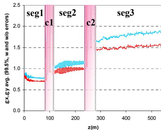
Figure 1: Transverse emittances of multi-charge state uranium beam w/o errors (red/dark) and with errors (blue/light) along the RIA driver linac.
