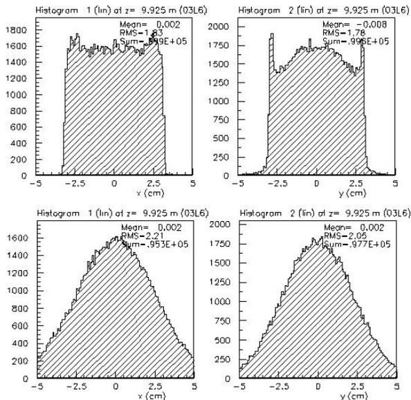
Figure 2: Effect of Octupoles on a Gaussian Beam Distribution. The Octupoles are turned off in the lower half of the figure.
