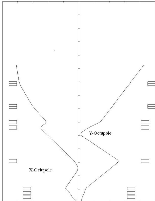
Figure 1: Beam Transport Envelope.
