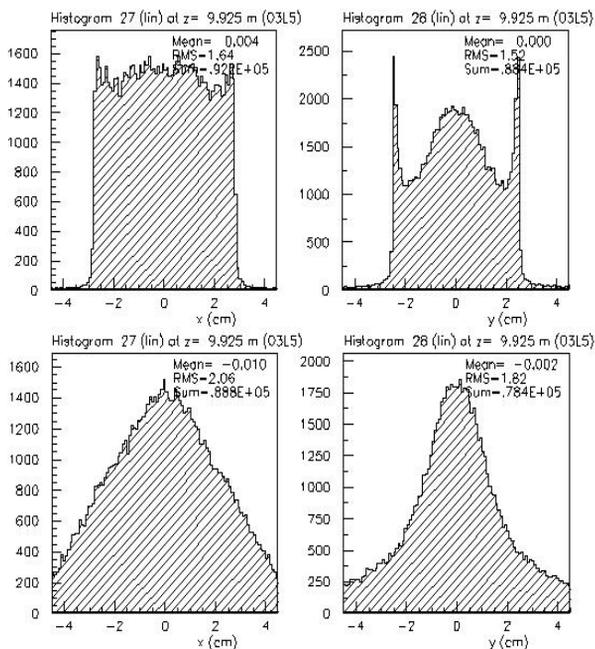
Figure 3: Effect of Octupoles on a Non-Gaussian Beam Distribution.
