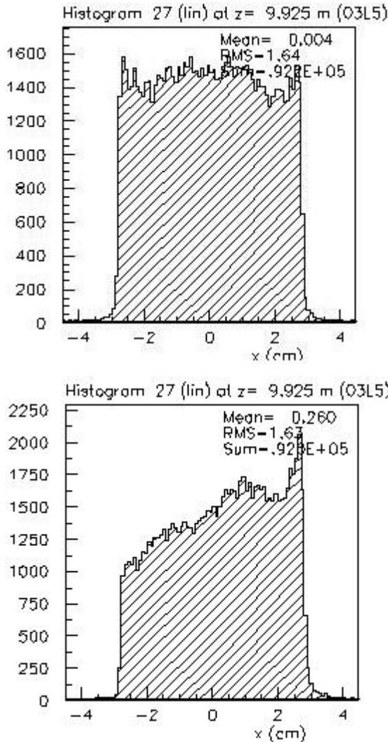
Figure 4: Effect on the horizontal beam profile by a 1mm horizontal displacement of Q2.
