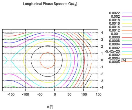
Figure 2: Longitudinal Phase Space for NSLS-II (analytical model:  $\alpha_1 = 1.7 \times 10^{-4}$ ,  $\alpha_2 = 1.4 \times 10^{-3}$ ).
