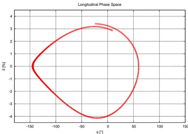
Figure 3: Longitudinal Phase-Space for NSLS-II (TRACY-2 with radiation).
