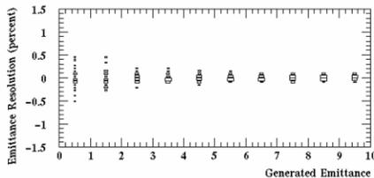
Figure 4: Emittance measurement with the offset removed.
