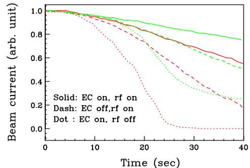
Figure 4: Comparison of lifetime that is simulated (in green) and measured (in red) for 400 MeV proton interacting with hydrogen pellet target of effective thickness of  $7.8 \times 10^{-9}$  g/cm<sup>2</sup>.
