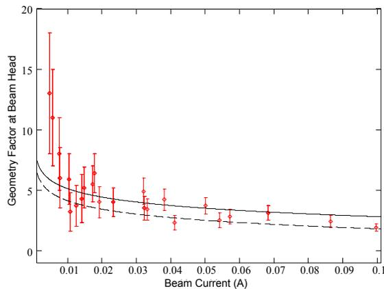
Figure 1: Geometry factor for beam head. Solid line is theoretical value with  $\alpha$  of one, dashed line is theoretical value with  $\alpha$  of zero.
