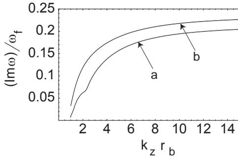
Figure 2: Plots of the normalized growth rate  $(Im\omega)/\omega_f$  versus  $k_z r_b$  for  $\bar{\nu}/\nu_0 = 0.3$ ,  $T_{||b}/T_{\perp b} = 0$  and  $m=0$  (curve a) and  $m=1$  (curve b).
