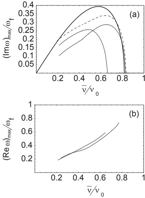
Figure 1: Plots of the normalized growth rate  $(Im\omega)_{max}/\omega_f$  and real frequency  $(Re\omega)_{max}/\omega_f$  at maximum growth versus normalized tune depression  $\bar{\nu}/\nu_0$  for  $T_{||b}/T_{\perp b} = 0$  and  $m=0$  (solid curve) and  $m=1$  (dotted curve). The thick solid curve corresponds to the simple estimate in Eq. (13).
