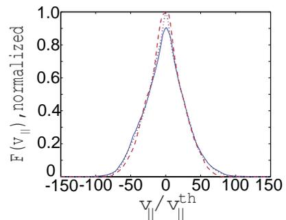
Figure 8: Plots of  $z$ -averaged longitudinal velocity distribution at times  $\omega_f t = 75$  (red dashed line),  $\omega_f t = 100$  (red dotted line) and  $\omega_f t = 150$  (solid blue line).
