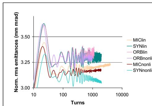
Figure 5:  $\epsilon_y$  for fully nonlinear lattice,  $Q_{0,x} = 6.19$  (compared with linearized AG).
