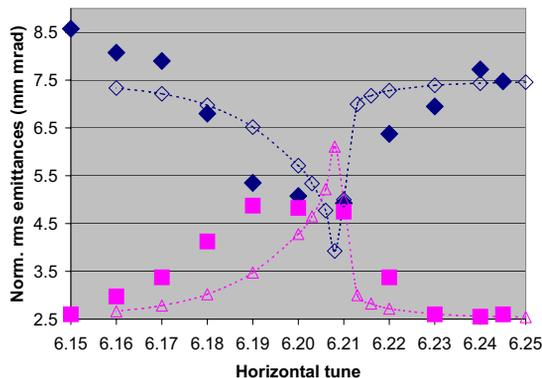
Figure 1: Final measured (full markers) and simulated (open markers) emittances as function of  $Q_{0,x}$ .
