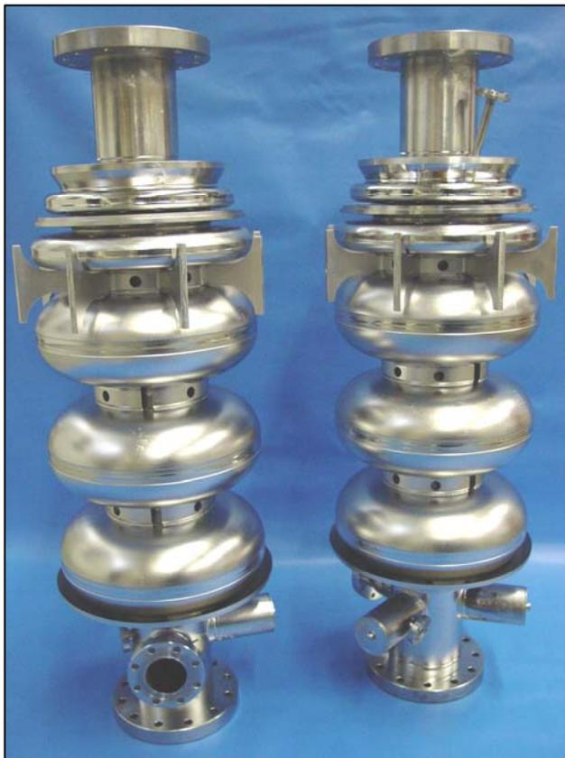
Figure 4: 3½ cell FZR SRF cavity.
