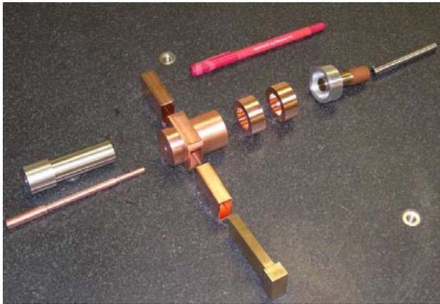
Figure 3: Low power model of the X-band normal conducting gun with the scale indicated by the red pen.
