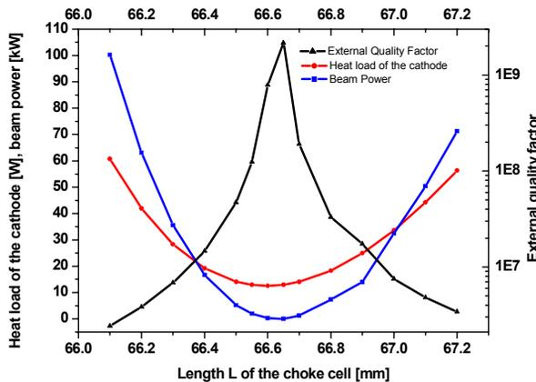
Figure 7: Dependence of beam power and heat load on the length of the choke filter.
