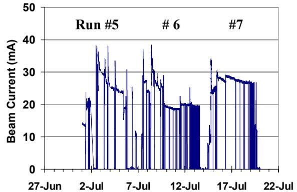
Figure 2: Average pulse current records for three experimental runs showing the best performance achieved using the original conditioning procedure.
