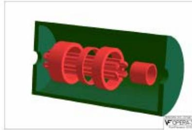
Figure 9: The OPERA-3D model of the MS-ECRIS (GYRO-SERSE) magnetic system. The first focusing solenoid is included in the main cryostat [9].
