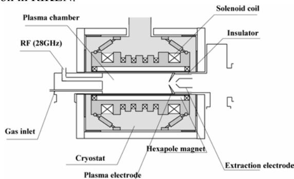
Figure 8: The new 28 GHz RIKEN ECRIS conceptual design with four small inner solenoid coils to have more control over the axial mirror field shape.
