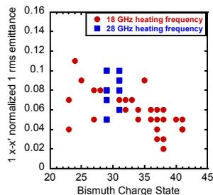
Figure 3: Dependence of the emittance value from the ion charge state for bismuth for the 18 GHz heated plasma and the 28 GHz heated plasma.
