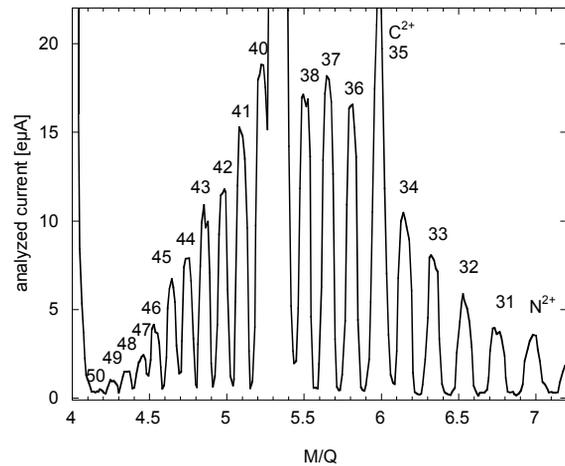
Figure 6: Analyzed Bi current for an ion source tune at 28 GHz optimized for  $Bi^{41+}$ .
