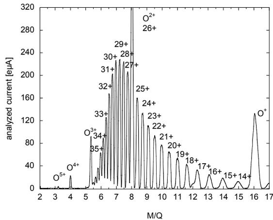
Figure 5: Analyzed Bi current for an ion source tune at 28 GHz optimized for  $Bi^{29+}$ .
