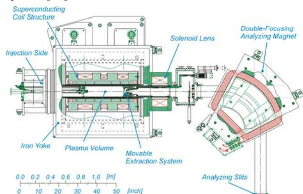
Figure 4: Mechanical layout of the beam transport system for VENUS.
