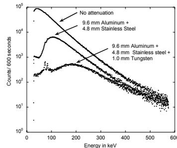
Figure 2: Axial bremsstrahlung spectra measured for 2 kW of 28 GHz microwave power on VENUS, using different materials as attenuator.
