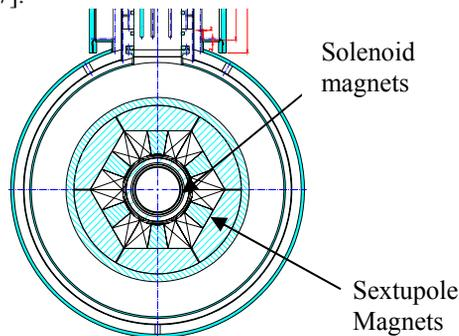
Figure 7 cross section view of the SECRAL source magnets at IMP, Lanzhou.
