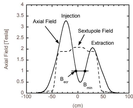
Figure 1: Typical magnetic fields used for VENUS for 28 GHz operation
