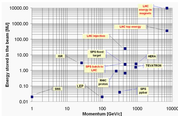
Figure 1: Stored beam energy as a function of the momentum for various accelerators. For comparison, 700 kJ are sufficient to heat and melt one kg copper.
