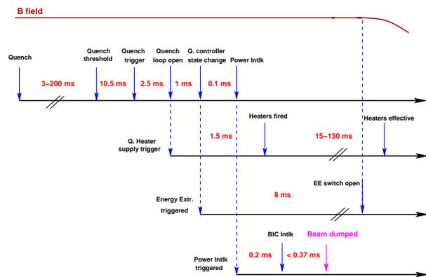
Figure 2: Time sequence of signals following a quench of a magnet until the beam is dumped, the quench heaters are fired and the energy is extracted from the circuit.
