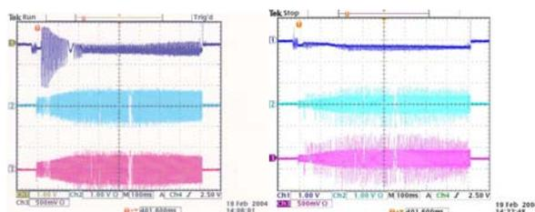
Figure 6 and 7: The top traces are phase detector signal between input and output gap voltage. The vertical scale is 9[degree/div]. The middle and bottom traces are cathode voltage and forward power respectively. The left plot is without and right is with feedforward beam loading compensation.
