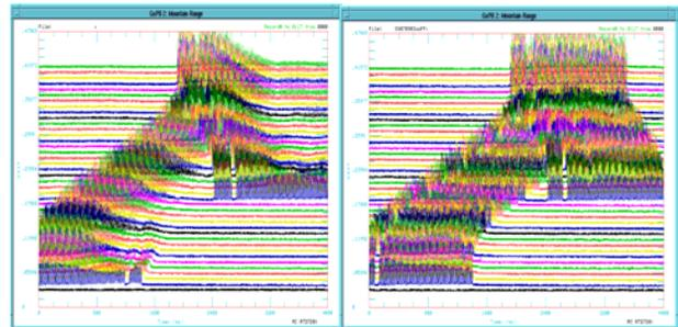
Figure 1 and 2: Mountain range plots of the WCM signal. The plots on the left and right show signal without and with feedforward beam loading compensation.
