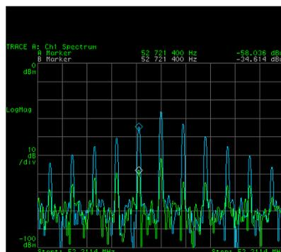
Figure 5: Frequency spectrums of gap voltage monitor on one of the eighteen cavities. Blue and green traces show signals without and with feedforward beam loading compensation. The vertical scale is 10dB/div.
