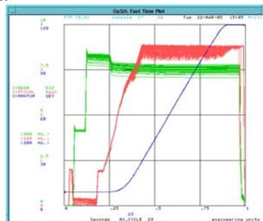
Figure 8: RFSUML: RF voltage[MV], MMNTUM: momentum[GeV/c], I:BEAM: total beam intensity [ $\cdot 10^{12}$  ppp]
