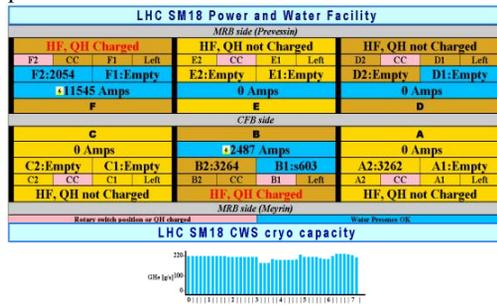
Figure 4: Power, Water & Helium flow [g/s]
