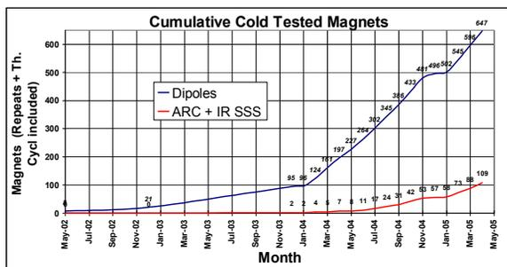
Figure 5: Cumulative Cold Tested magnets.
