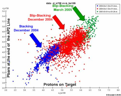
Figure 8. The amount of antiprotons produced as a function of proton beam on the antiproton production target.
