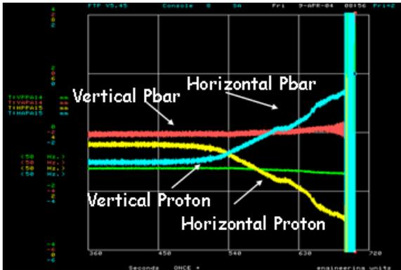
Figure 12. Tevatron BPM signals as the Tevatron helix is opened.
