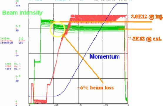
Figure 7. Main Injector intensity profile of slip stacking.
