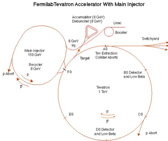
Figure 1. Layout of the Fermilab collider complex
