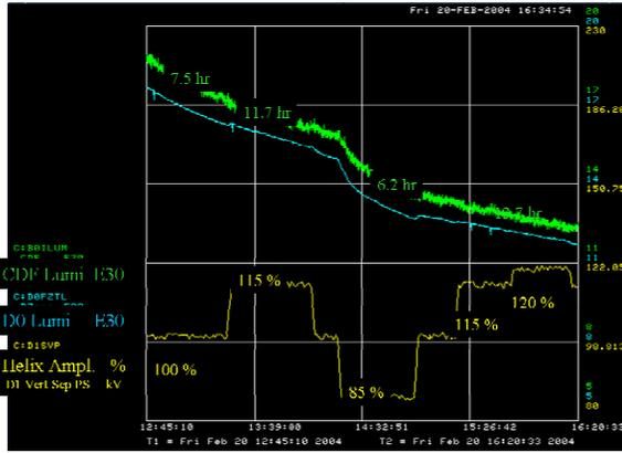
Figure 11. Luminosity lifetime as a function of the helix separation.
